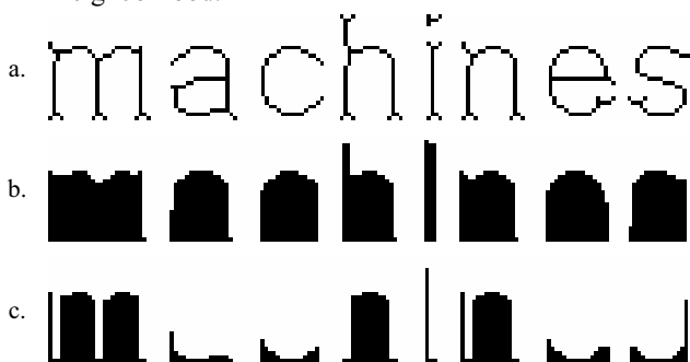
Figure 3. A visual representation of the Top-Bottom Shape Projections: (a) Original Image. (b) Top Shape Projection. (c) Bottom Shape Projection
